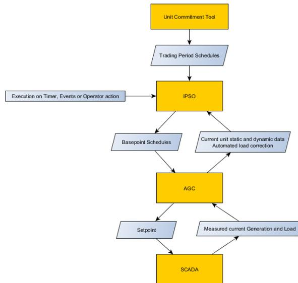
Figure 3: High level IPSO interactions
