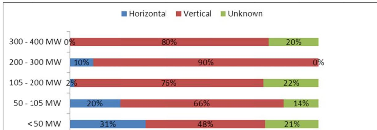
Figure 5: 12 Share of unit axis depending on the unit power output (MW) (Alstom, 2013)
